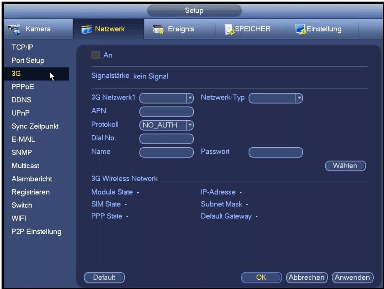
The screenshot shows the 'Setup' interface with the 'Netzwerk' (Network) tab selected. The left sidebar contains a list of settings: Kamera, Netzwerk, Ereignis, SPEICHER, and Einstellung. Under 'Netzwerk', the following options are listed: TCP/IP, Port Setup, 3G (highlighted), PPPoE, DDNS, UPnP, Sync Zeitpunkt, E-MAIL, SNMP, Multicast, Alarmbericht, Registrieren, Switch, WIFI, and P2P Einstellung.
